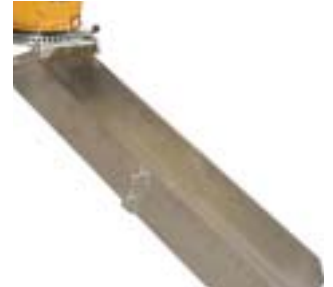
Extended chute for high lorry
